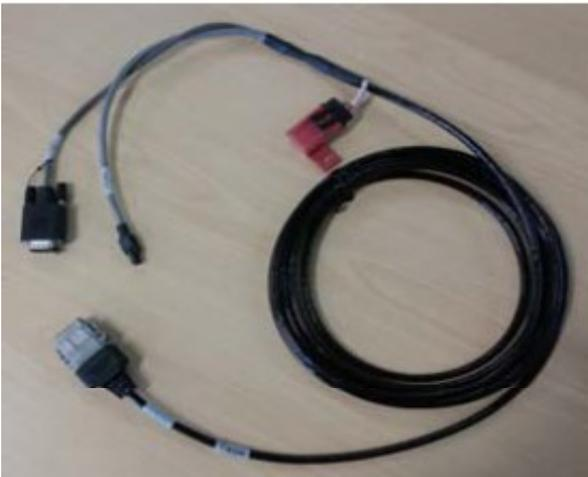
The custom harness allows the GX-450/372 cable to be plugged into the display for power AND signal and does not require the use of the USB port
